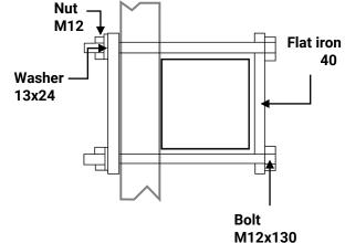
**NOTE!** A torque wrench must be used during assembly.
