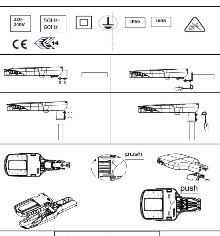
Make sure the clips are properly pushed togheter when mounted
