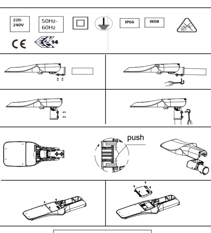
Make sure the clips are properly pushed togheter when mounted
